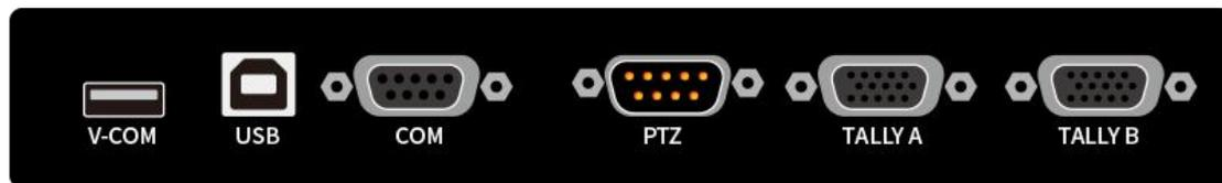
**V-COM/COM:** update the switch platform panel use, need connect the USB joggle when update the system.
